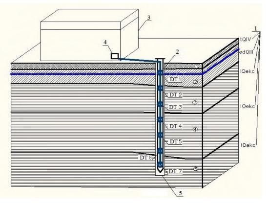
Figure 2. The plan diagram of the installation of temperature sensors in the exploratory well.
